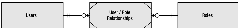
Figure 5-1. Simple entity relationship diagram for storing users, roles, and role assignments in a database
